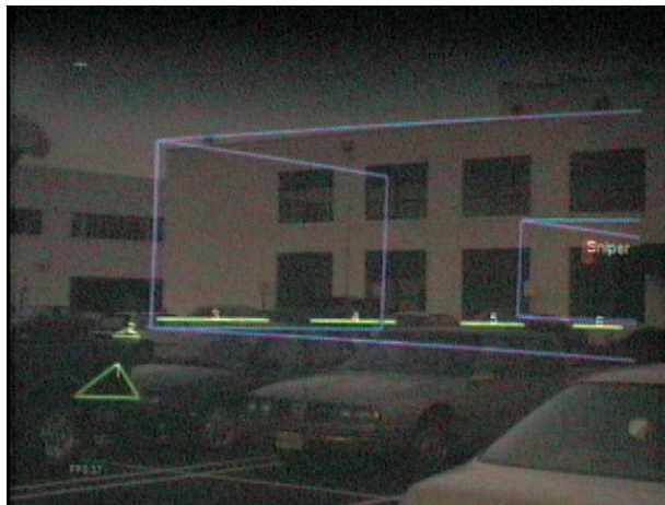
Figure 2: Sample output from the prototype augmented reality system. In this scenario, a user follows a route (triangles) around the edge of a building. Sniper is visible beyond.
