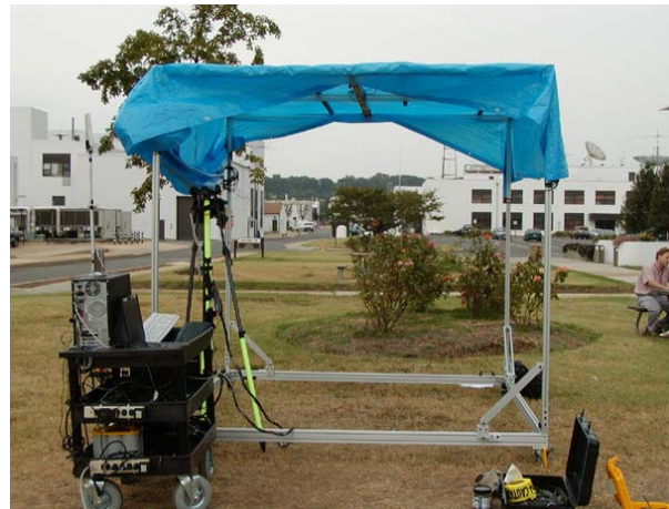
Figure 6. Outdoor tracking cage setup for BARS formative evaluation study. The cage has overhead tracking rails (barely visible under the blue canopy) so that the augmenting graphics can change as a user moves around.
