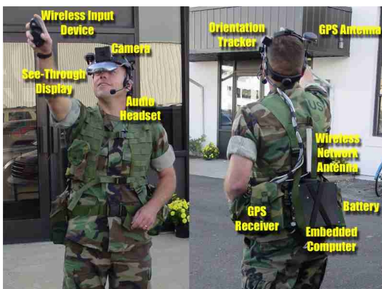
Figure 1: A prototype implementation of BARS using commercially available components. The wearable computer produces graphics seen in the display. Audio and wireless hand-held devices are used to interact with the system.
