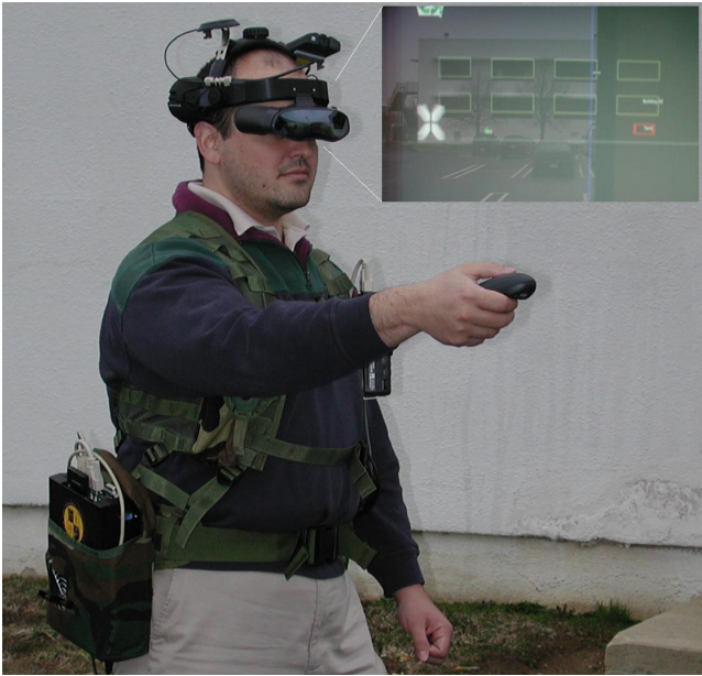
Figure 2: A user wearing our system. The inset right shows a generic view of virtual spatial data aligned with the real environment.
