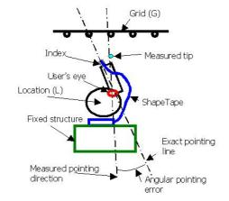
Figure 3: Overhead View of the Pointing Experiment
